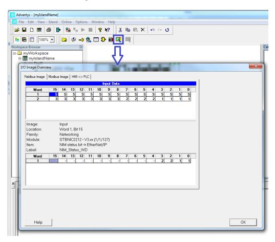
Here 2 input words and 1 output word are exchanged. Click on bits to display the corresponding description.
